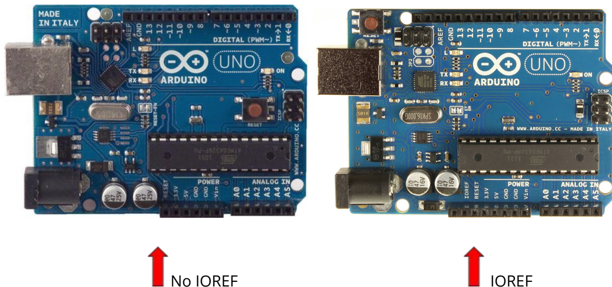
Figure 2. Arduino UNO header without (left) and with (right) IOREF PIN.
